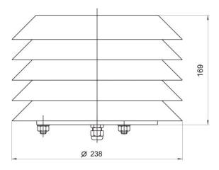
Met Cover 3 B - Ground Shield – designated for shielding of sensors near ground . Needles in bottom part serves for fixation of shield in terrain
