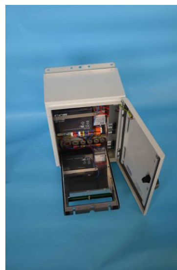
Back panel with power supply components (front panel is tilted)
